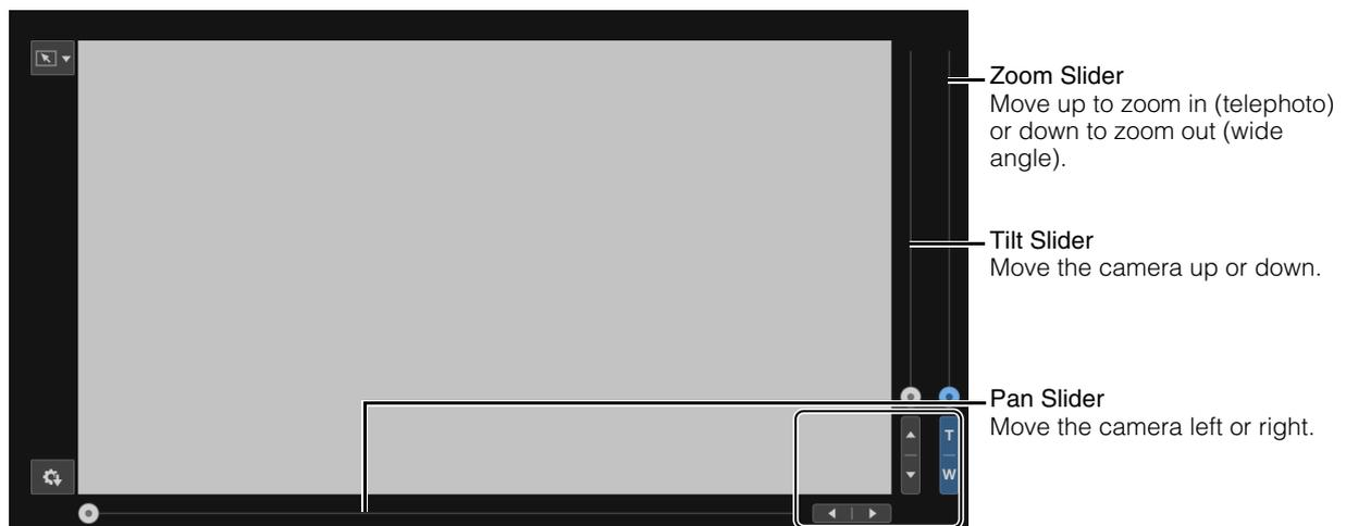
Fine tune the pan, tilt, and zoom positions by clicking the ◀ or ▶, ▲ or ▼, or T or W buttons.
