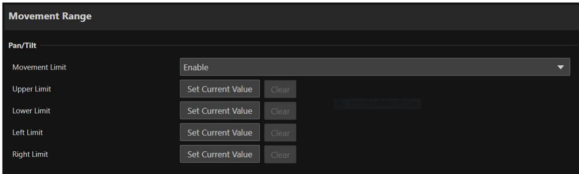
The screenshot shows a dark-themed settings window titled "Movement Range". Under the "Pan/Tilt" section, there is a "Movement Limit" dropdown menu currently set to "Enable". Below this, there are four rows of controls for "Upper Limit", "Lower Limit", "Left Limit", and "Right Limit". Each row contains a "Set Current Value" button and a "Clear" button. A "Save" button is located at the bottom right of the settings area.
